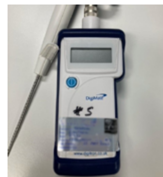
Figure 9. Example of a calibrated temperature probe
