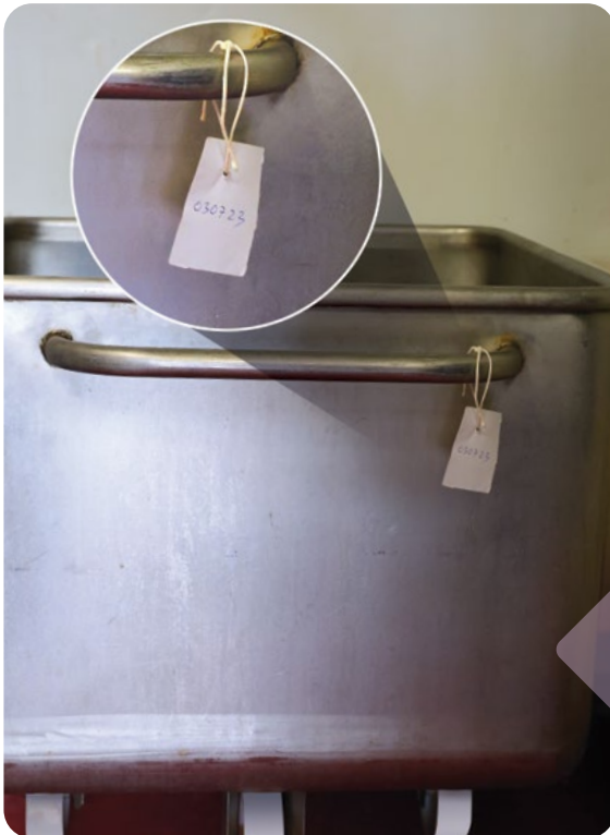
An example of an internal traceability tag identifying a product batch.
